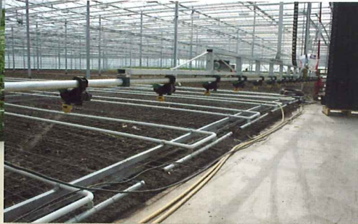
Computer controlled spraying mechanisms mean there's no human contact with pesticides.
