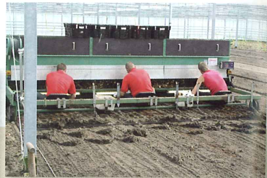
One way of helping workers at Lilies of Life is through the use of this bulb planting machine that does away with back-breaking work by allowing workers to sit comfortably whilst planting. No heavy lifting is needed.
